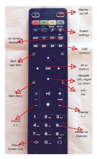
The top RED on off button turns box between standby and on. We recommend not disconnecting the power every night, leave on standby. The box will automatically go to standby when not in use.
